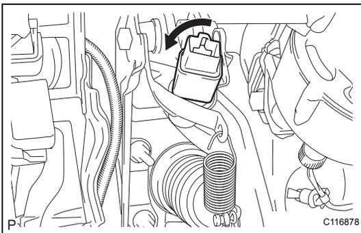
**19. REMOVE STOP LIGHT SWITCH MOUNTING ADJUSTER**
