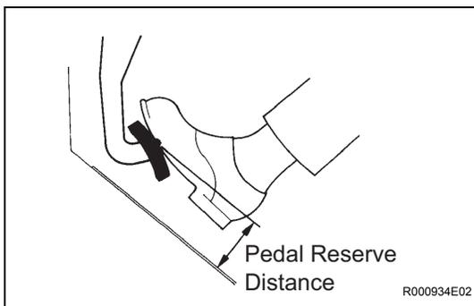
(8) Check the stop light switch clearance.
