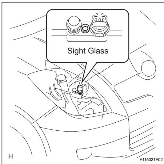
(a) Check the sight glass of the cooler unit refrigerant liquid pipe.
