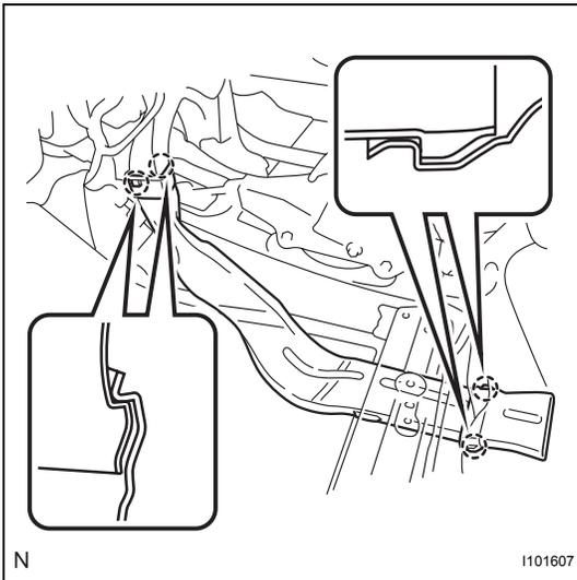
**60. REMOVE REAR NO. 2 AIR DUCT (for Cold Area Specification Vehicles)**
