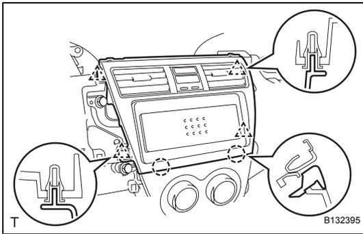
5. **INSTALL INSTRUMENT CLUSTER FINISH PANEL CENTER SUB-ASSEMBLY**
