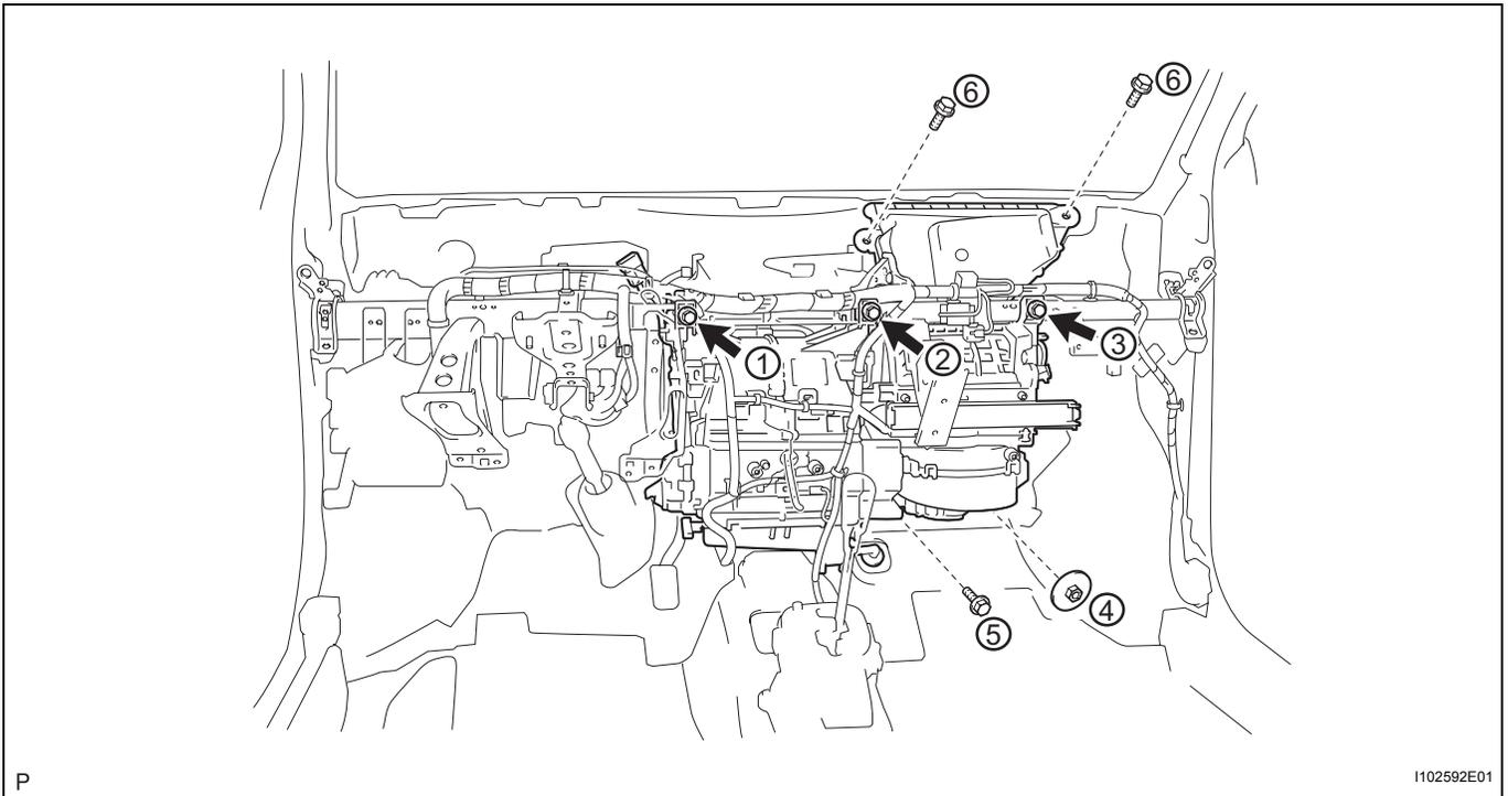
(d) Install the wire harness with the clamps and connect the connectors.
