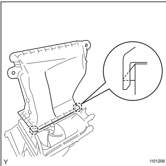
**6. INSTALL NO. 1 AIR DUCT SUB-ASSEMBLY**
