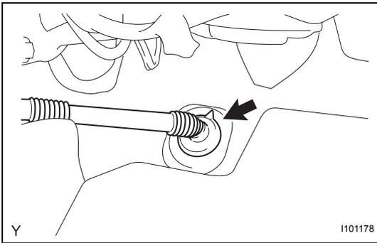
(b) Remove the bolt and disconnect the ground wire.
