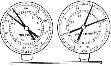
NOTE: These gauge indications occur when the refrigeration system opens and the refrigerant is supplied without performing vacuum purging.
