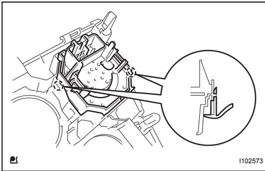
(b) Engage the 2 claws and install the heater control.
