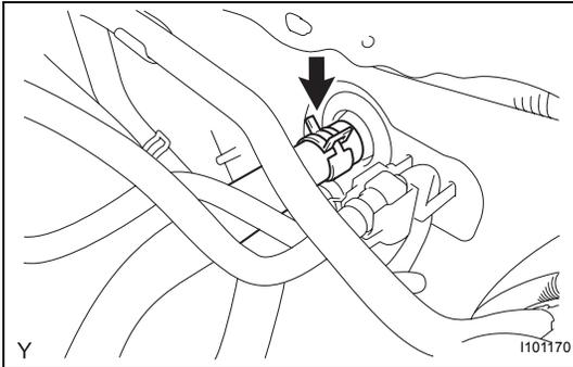
**15. DISCONNECT HEATER WATER OUTLET HOSE A (FROM HEATER UNIT)**
