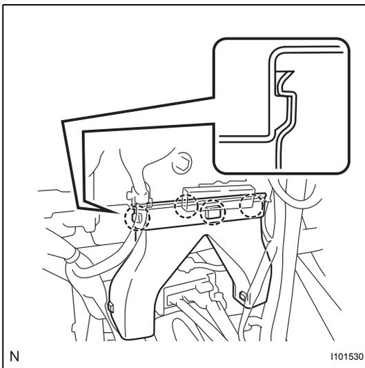
**69. REMOVE REAR NO. 3 AIR DUCT (for Cold Area Specification Vehicles)**
