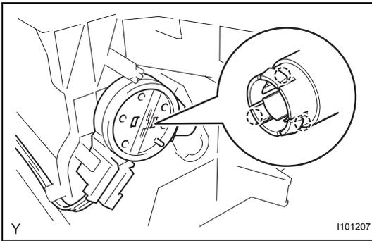
**2. REMOVE AIR INLET DAMPER CONTROL CABLE SUB-ASSEMBLY**
