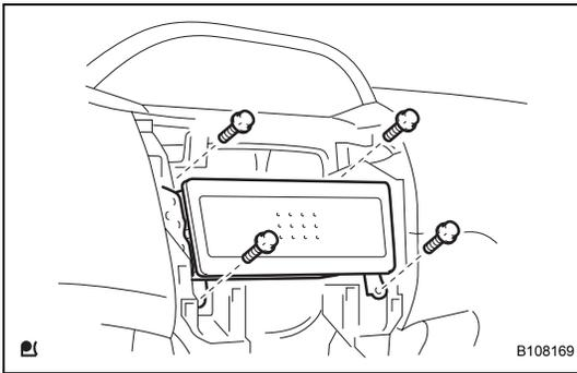
51. **INSTALL RADIO TUNER OPENING COVER (w/o Radio Receiver)**
