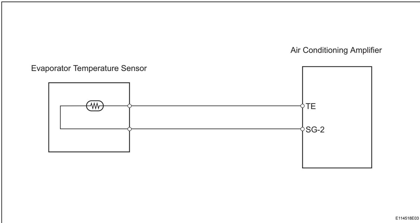
**INSPECTION PROCEDURE****1****READ VALUE USING INTELLIGENT TESTER (EVAP FIN TEMP)**
