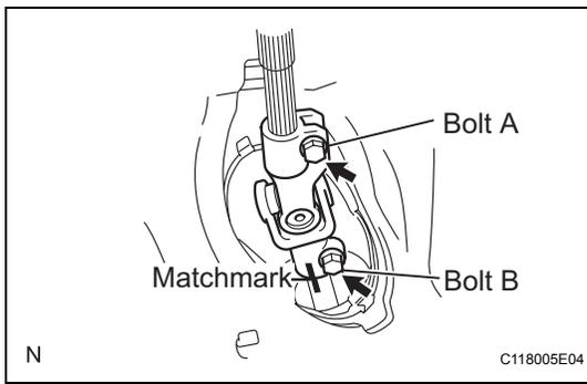
16. **INSTALL STEERING SLIDING YOKE SUB-ASSEMBLY**
