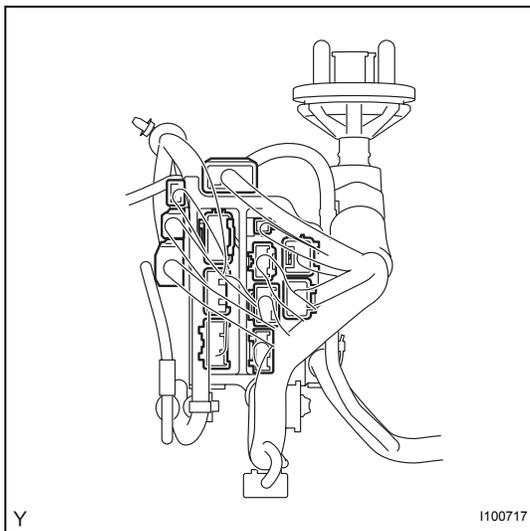
(b) Disconnect the connectors and separate the connector No. 2 holder.
