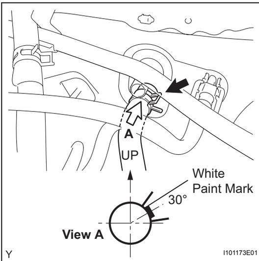
59. **CONNECT HEATER WATER OUTLET HOSE A (FROM HEATER UNIT)**
