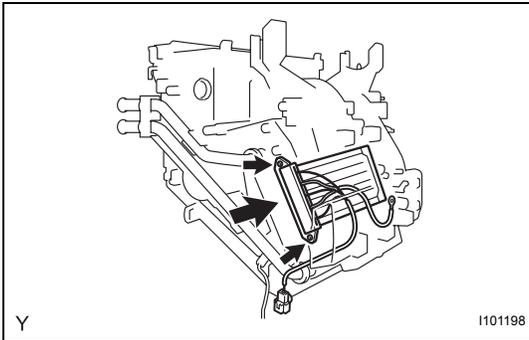
**5. INSTALL PTC HEATER ASSEMBLY (for Cold Area Specification Vehicles)**
