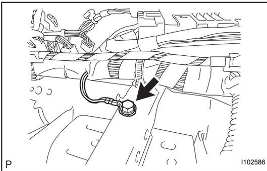
(f) Install the ground wire with the bolt.
