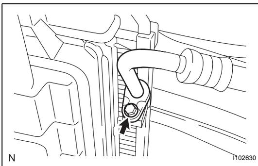
10. DISCONNECT LIQUID TUBE SUB-ASSEMBLY A
