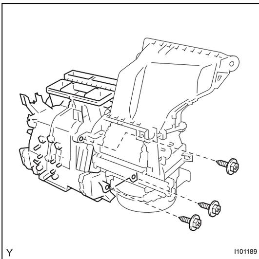
**2. INSTALL AIR CONDITIONING AMPLIFIER ASSEMBLY**
