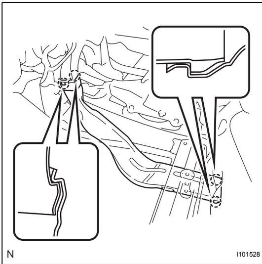
**9. INSTALL REAR NO. 2 AIR DUCT (for Cold Area Specification Vehicles)**
