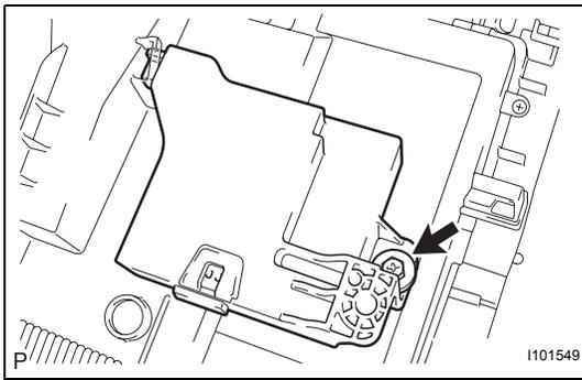
**67. REMOVE AIR CONDITIONING AMPLIFIER ASSEMBLY**
