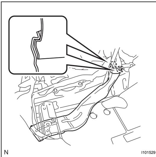
**68. REMOVE REAR NO. 1 AIR DUCT (for Cold Area Specification Vehicles)**
