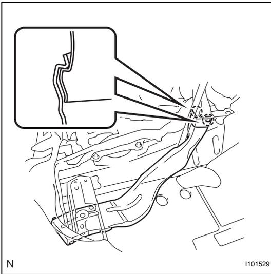
**61. REMOVE REAR NO. 1 AIR DUCT (for Cold Area Specification Vehicles)**
