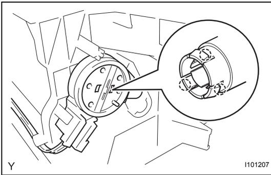
**5. INSTALL AIR INLET DAMPER CONTROL CABLE SUB-ASSEMBLY**
