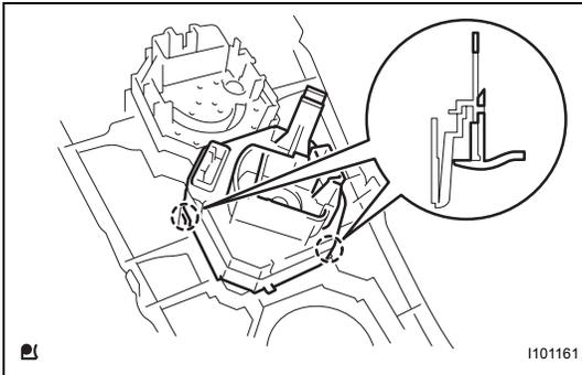
(b) Engage the 2 claws and install the heater control base.
