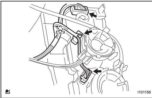
(b) Disconnect the 3 connectors and the clamp.
