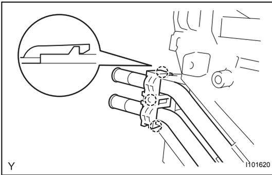
(b) Engage the 3 clips and install the clamp.
