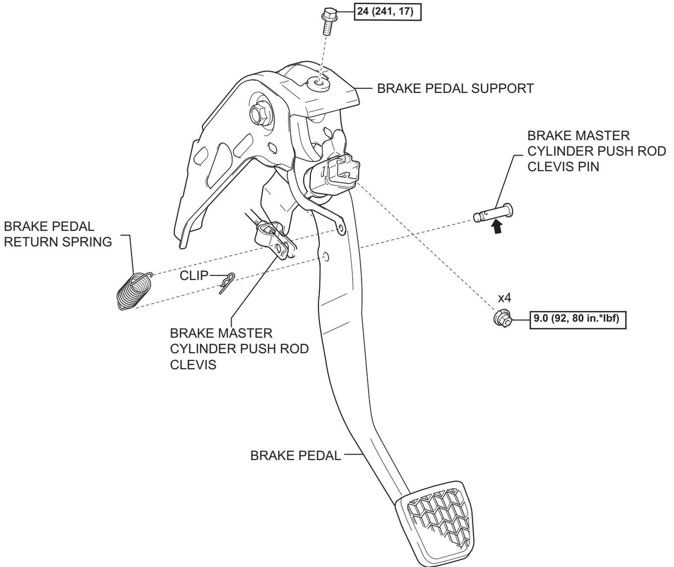
$\boxed{\text{N}^*\text{m (kgf}^*\text{cm, ft.}^*\text{lbf)}}$  : Specified torque
