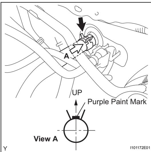
60. **INSTALL LIQUID TUBE SUB-ASSEMBLY**
