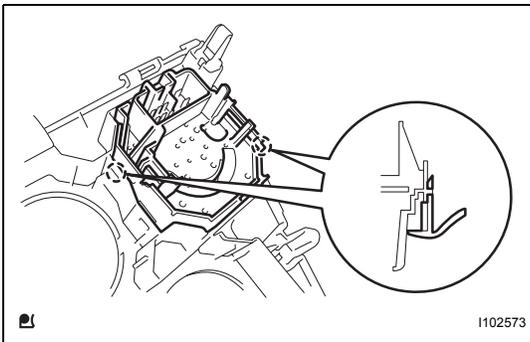
**3. REMOVE HEATER CONTROL SUB-ASSEMBLY**
