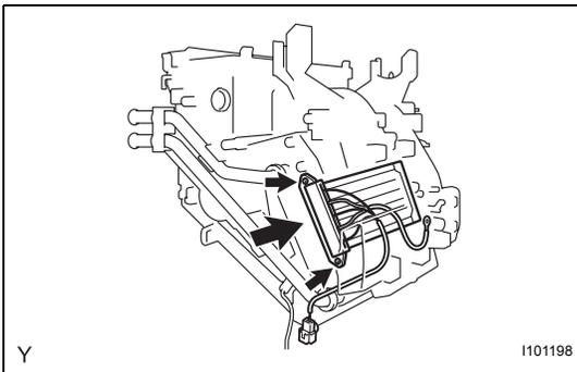
**5. REMOVE PTC HEATER ASSEMBLY (for Cold Area Specification Vehicles)**
