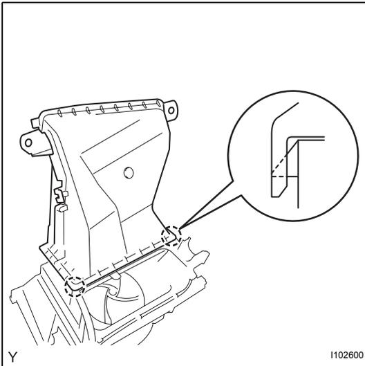
2. REMOVE AIR INLET DAMPER CONTROL CABLE SUB-ASSEMBLY
