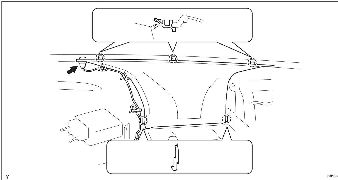
**67. REMOVE REAR NO. 2 AIR DUCT (for Cold Area Specification Vehicles)**
