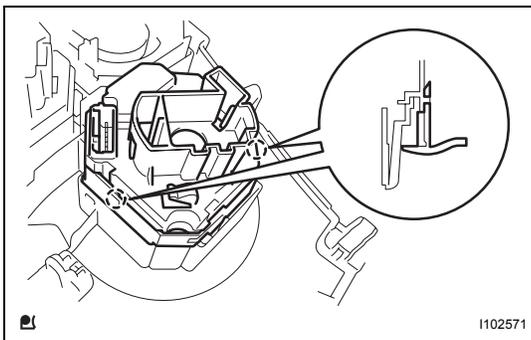
(b) Engage the 2 claws and install the No. 3 heater control knob.
