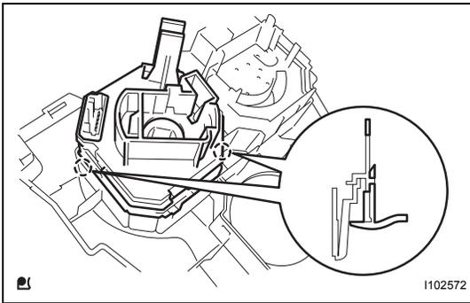
**2. REMOVE HEATER CONTROL BASE SUB-ASSEMBLY**
