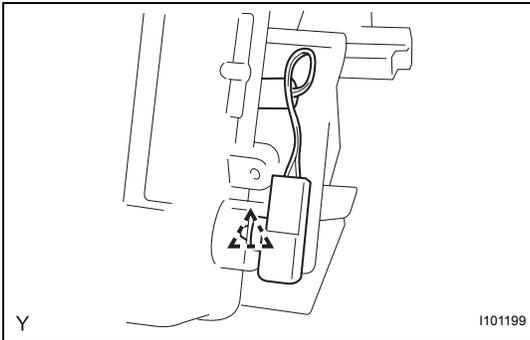
**7. REMOVE NO. 1 COOLER EVAPORATOR SUB-ASSEMBLY**
