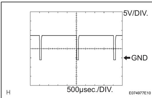
(c) Waveform 3 (Reference) : Using an oscilloscope
