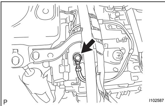
(g) Install the ground wire with the bolt. (for Cold area specification vehicles)
