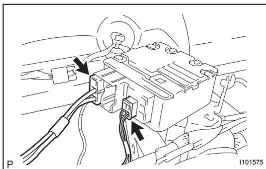
(h) Install the ground wire with the bolt.
