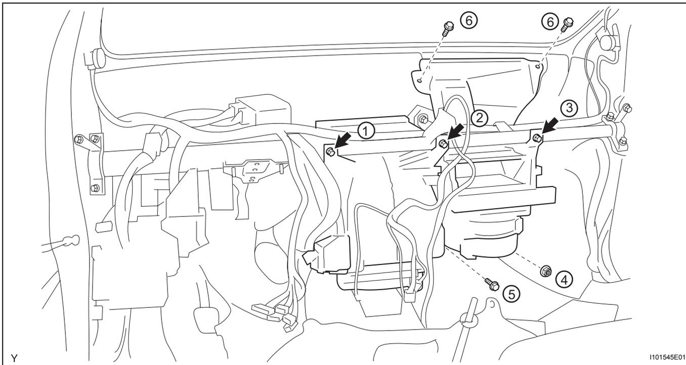
(e) Install the wire harness with the clamps and connectors.
