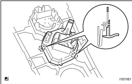
**2. REMOVE HEATER CONTROL BASE SUB-ASSEMBLY**
