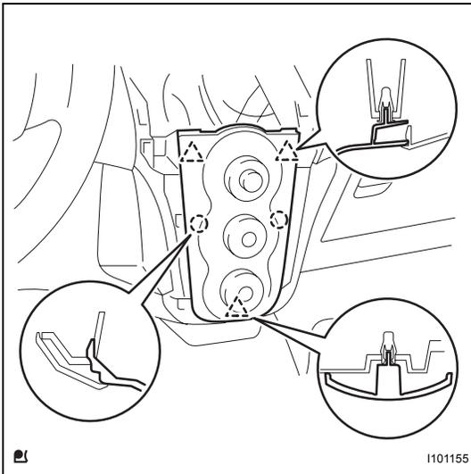
(b) Engage the 3 clips and 2 claws and install the air conditioning panel.
