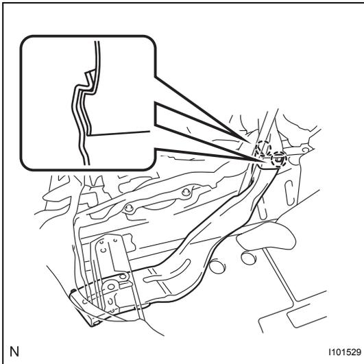
**8. INSTALL REAR NO. 1 AIR DUCT (for Cold Area Specification Vehicles)**
