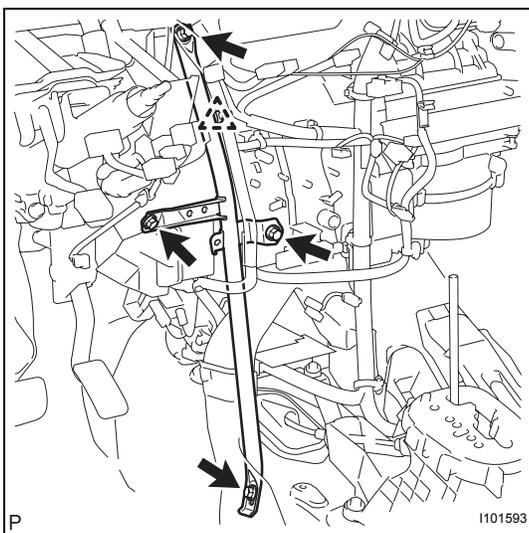
**70. REMOVE INSTRUMENT PANEL BRACE SUB-ASSEMBLY**
