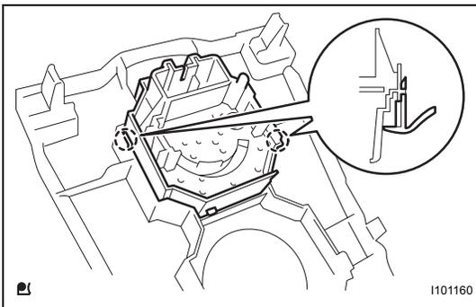
**3. REMOVE HEATER CONTROL SUB-ASSEMBLY**
