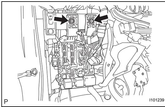
(b) Remove the 2 bolts and separate the main body ECU.
