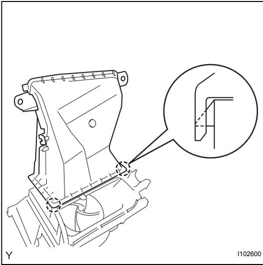
**6. INSTALL NO. 1 AIR DUCT SUB-ASSEMBLY**
