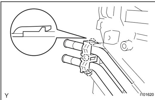
**6. REMOVE HEATER RADIATOR UNIT SUB-ASSEMBLY**
