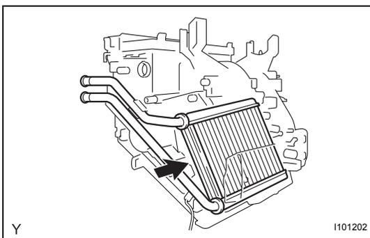
**4. INSTALL HEATER RADIATOR UNIT SUB-ASSEMBLY**
