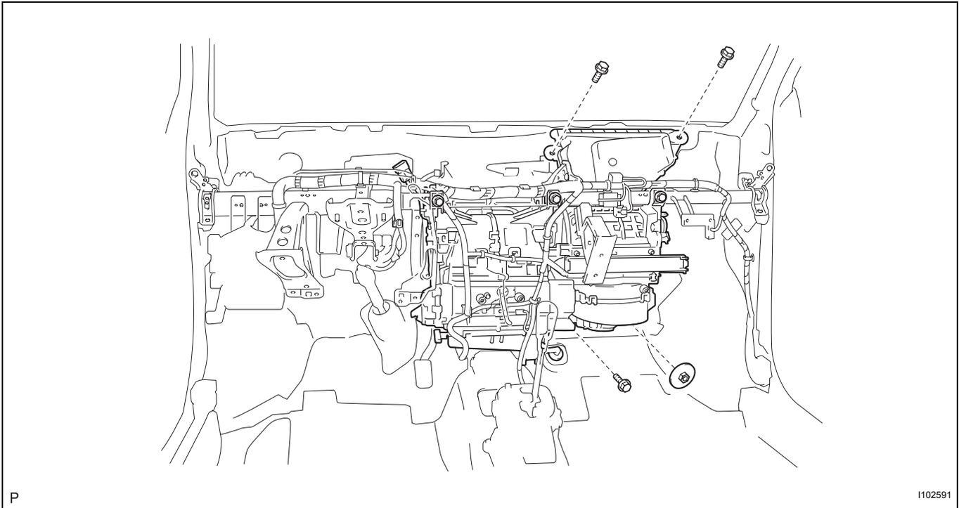
(h) Remove the 9 bolts and remove the instrument panel reinforcement together with the air conditioning unit.
