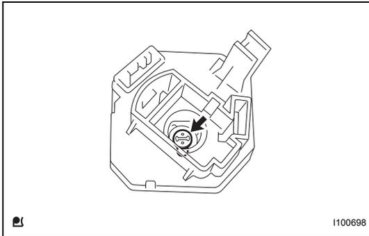
**2. INSTALL HEATER CONTROL BASE SUB-ASSEMBLY**
