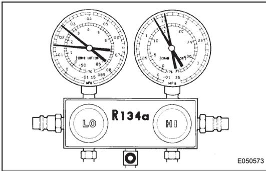
(1) When the refrigerant volume is correct, the gauge reading indicates as follows:
