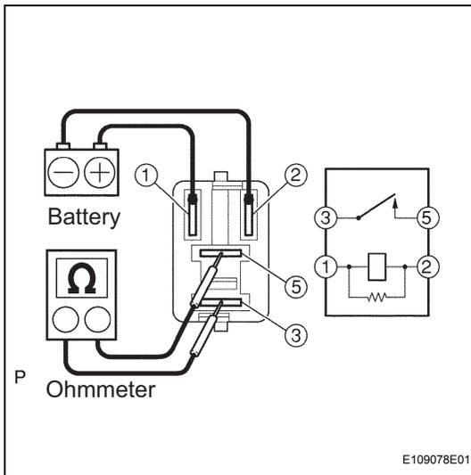
If the result is not as specified, replace the PTC heater relay.
