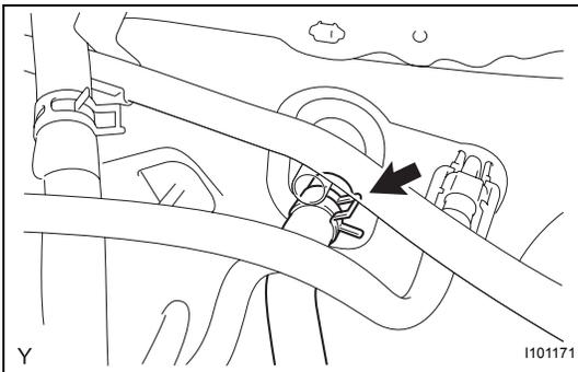
**16. DISCONNECT HEATER WATER INLET HOSE A**
