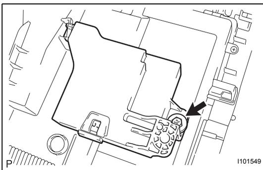
**3. INSTALL INSTRUMENT PANEL REINFORCEMENT**
