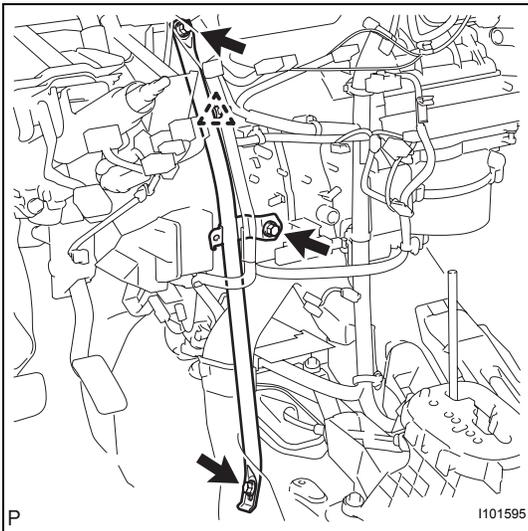
**63. REMOVE INSTRUMENT PANEL BRACE SUB-ASSEMBLY**
