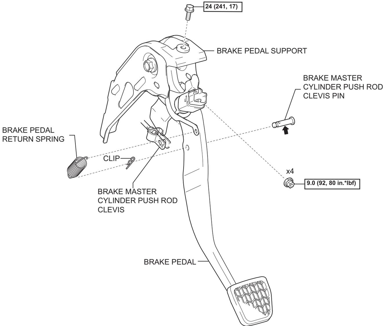
$\boxed{\text{N}^*\text{m (kgf}^*\text{cm, ft.}^*\text{lbf)}}$  : Specified torque
