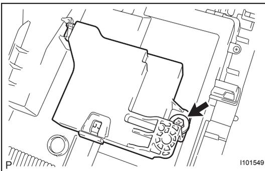
**2. INSTALL AIR CONDITIONING AMPLIFIER ASSEMBLY**
