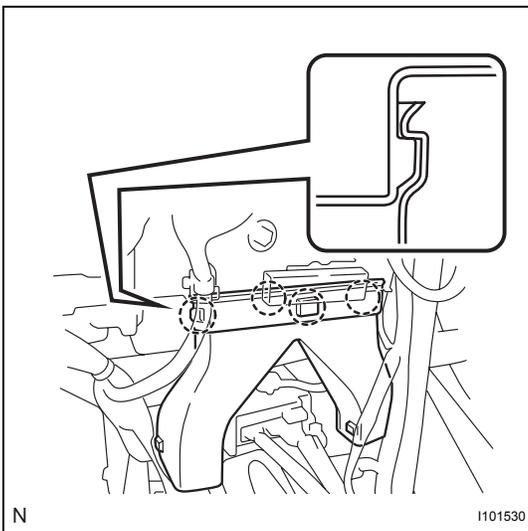
**62. REMOVE REAR NO. 3 AIR DUCT (for Cold Area Specification Vehicles)**
