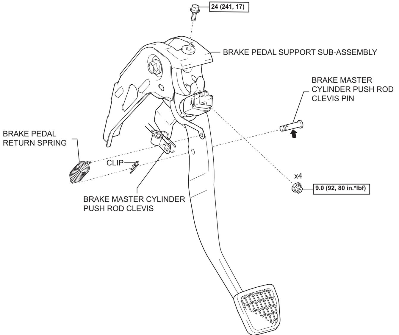
$\boxed{\text{N}^*\text{m (kgf}^*\text{cm, ft.}^*\text{lbf)}}$  : Specified torque
