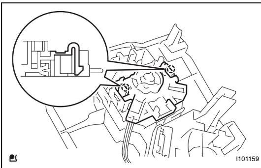
**9. DISCONNECT AIR INLET DAMPER CONTROL CABLE SUB-ASSEMBLY**
