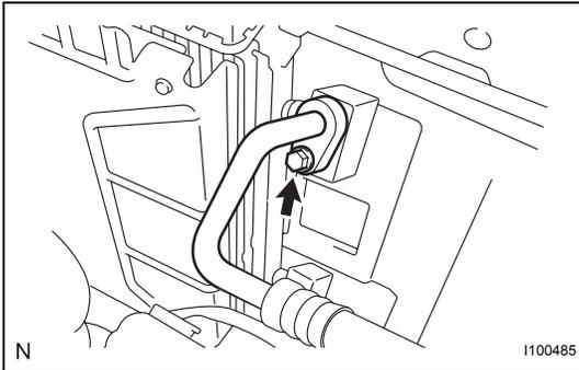
10. DISCONNECT LIQUID TUBE SUB-ASSEMBLY A
