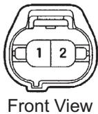
(a) Disconnect the C20 ECM connector and the C3 purge VSV connector.
