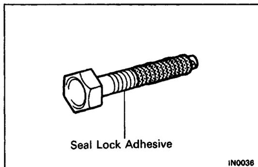
6. Precoated parts are bolts and nuts, etc. that are coated with a seal lock adhesive at the factory.
