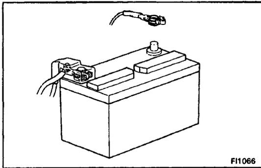
1. Malfunction symptoms of the airbag system are difficult to confirm, so the diagnostic codes become the most important source of information when troubleshooting. When troubleshooting the airbag system, always inspect the diagnostic codes before disconnecting the battery (See page [AB-25](#)).
