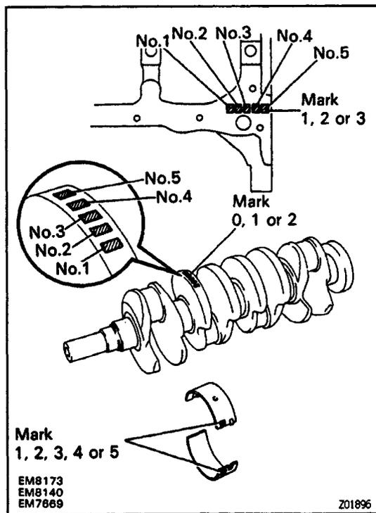
**HINT:** If replacing the cylinder block subassembly, the bearing standard clearance will be:
