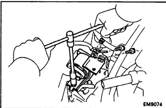
(b) Remove the through bolt, nut, three bolts and LH mounting insulator.
