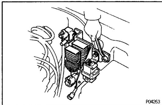
**16. DISCONNECT A/C IDLE-UP VALVE, AND REMOVE SOLENOID RESISTOR ASSEMBLY**
