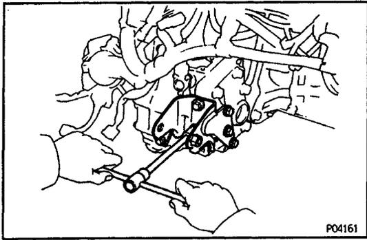
**41. REMOVE REAR ENGINE MOUNTING BRACKET**
