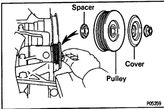
(f) Remove the nut, pulley cover, idler pulley and spacer.
