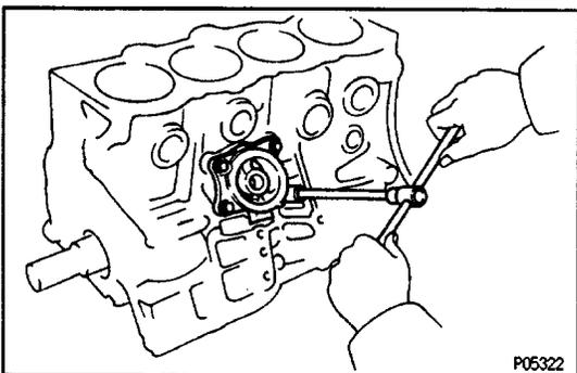
(c) Install the oil cooler bracket with the four bolts.
