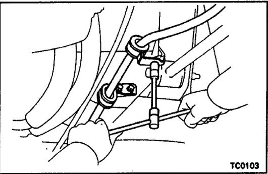
(j) Install the parking brake cable with the two clamp and three bolts.
