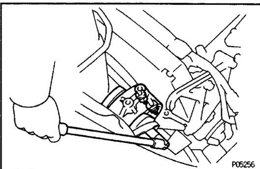
(c) Remove the through bolt, two nuts and RH mounting insulator.
