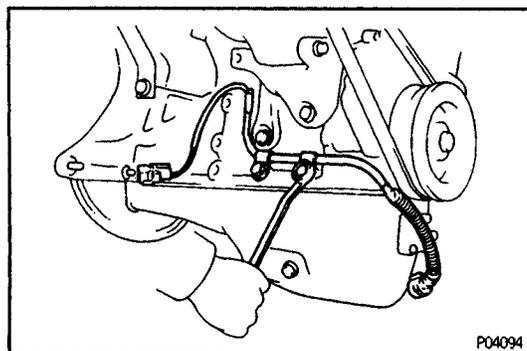
(b) Remove the two bolts and sensor wire.
