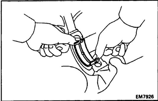
(b) Align the bearing claw with the claw groove of the main bearing cap, and push in the five lower bearings.
