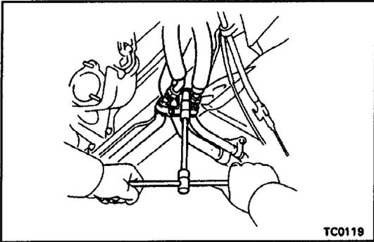
(h) Install the A/C pipes with the two clamps and nut.
