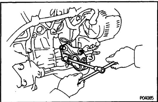
(b) Remove the two bolts and bearing bracket.
