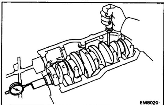
**5. CHECK CRANKSHAFT THRUST CLEARANCE**
