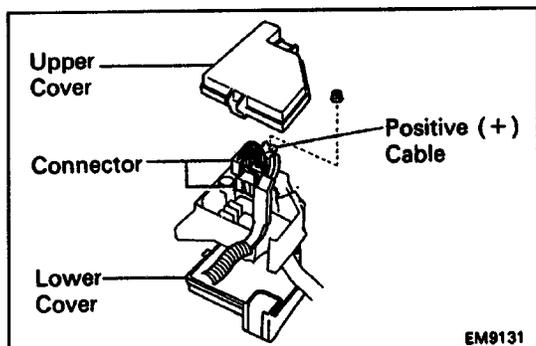
(b) Remove the upper and lower covers from the relay box.
