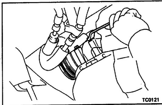
(i) Remove the two bolts, and disconnect the A/C compressor from the engine.
