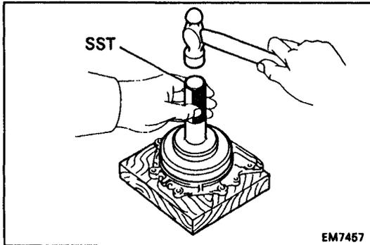
(b) Using SST and a hammer, tap in a new oil seal until its surface is flush with the rear oil seal edge.
