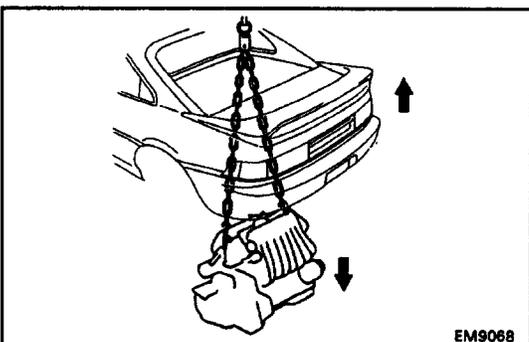
(d) Lower the engine out of the vehicle slowly and carefully, and raise the vehicle.
