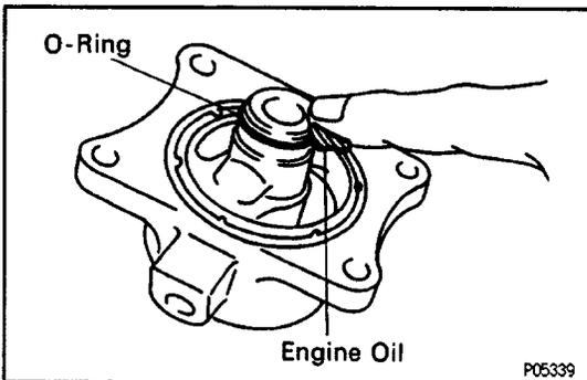
(b) Apply a light coat of engine oil on the small O-ring.
