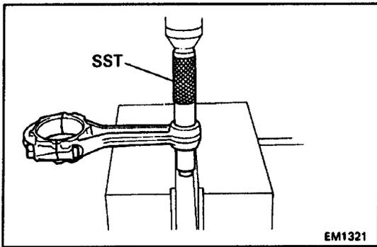
**C. If necessary, replace connecting rod bushing**
