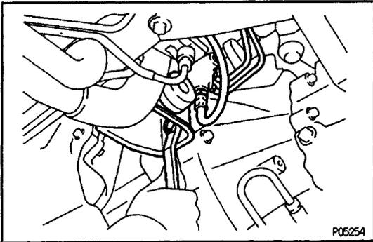
(b) Remove the two bolts and mounting bracket. Disconnect the clutch release cylinder from the transaxle.
