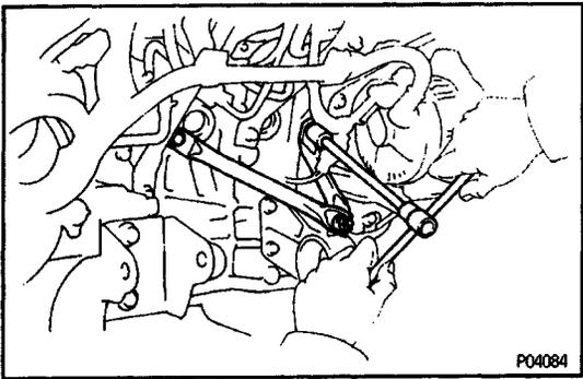
**43. REMOVE DRIVE SHAFT BEARING BRACKET**
