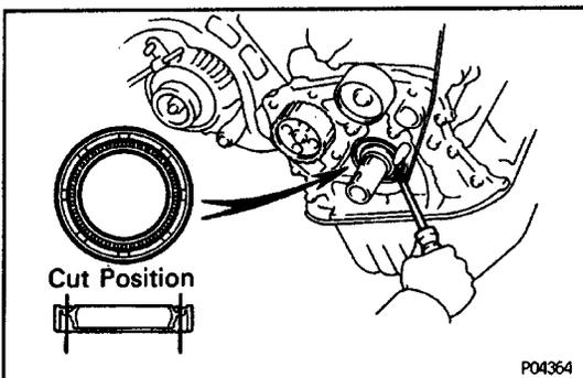
(c) Apply MP grease to a new oil seal lip.
