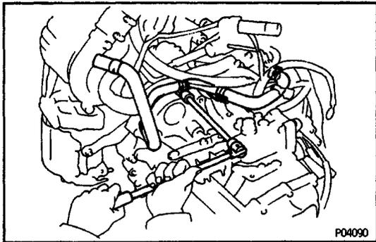
**6. REMOVE HEATER WATER PIPE**
