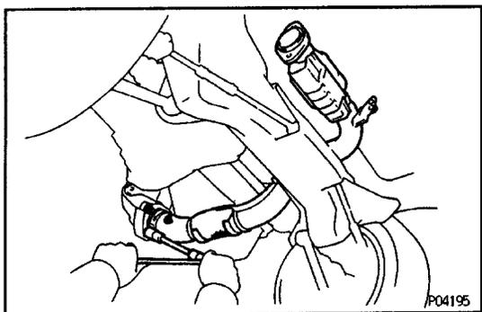
(c) Using a 14 mm deep wrench, remove the three nuts.
