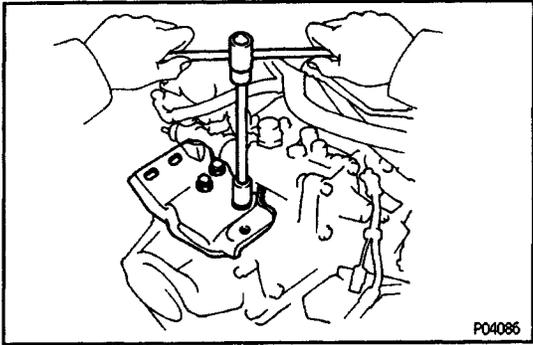
**42. REMOVE LH ENGINE MOUNTING BRACKET**
