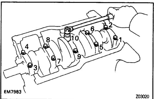
**6. REMOVE MAIN BEARING CAPS AND CHECK OIL CLEARANCE**
