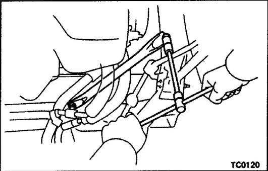
(i) Install the lower suspension brace with the two bolts.
