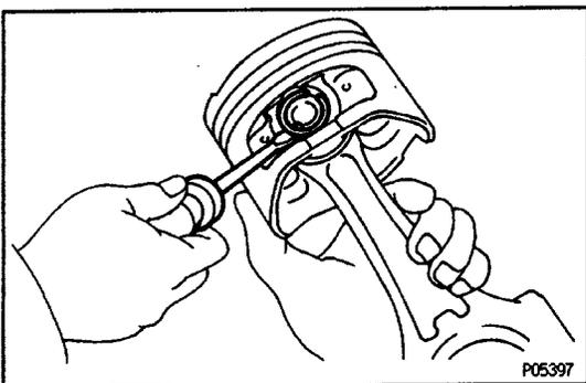
(e) Using a small screwdriver, Install a new snap ring on the other side of the piston pin hole.
