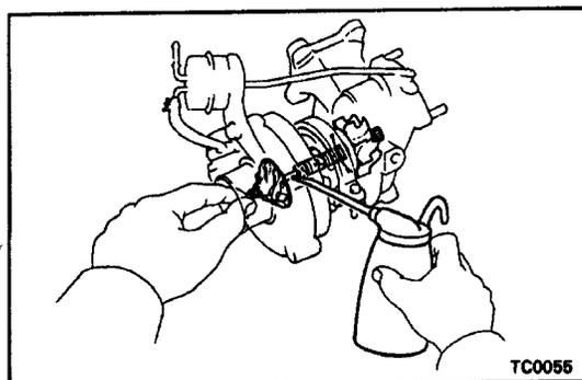
5. Use caution when removing and reinstalling the turbocharger assembly. Do not drop it or bang it against anything or grasp it by easily-deformed parts, such as the actuator or rod, when moving it.
