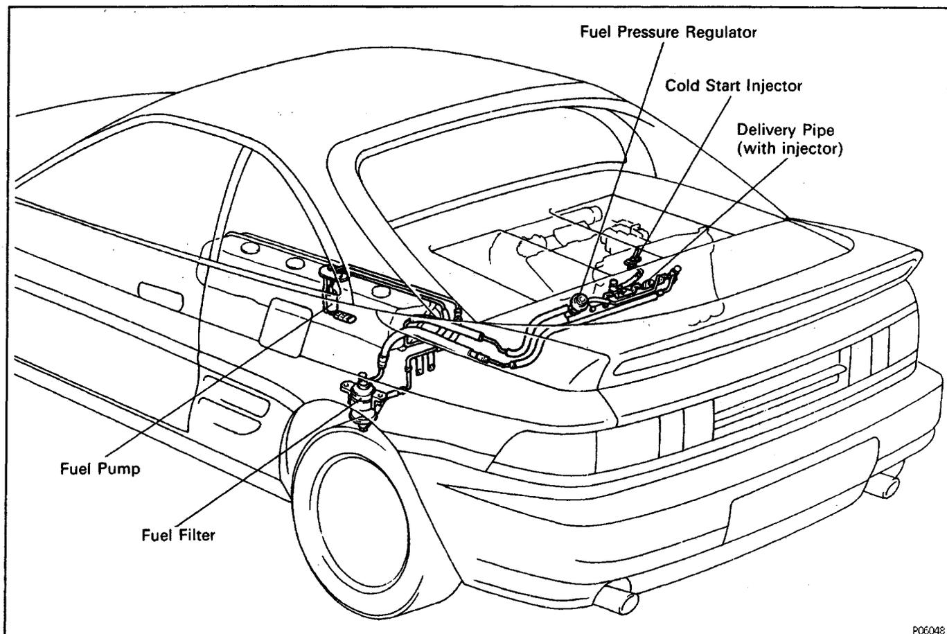
Fuel is pumped up by the fuel pump, flows through the fuel filter and is distributed to each injector and cold start injector at a set pressure maintained by the pressure regulator.
