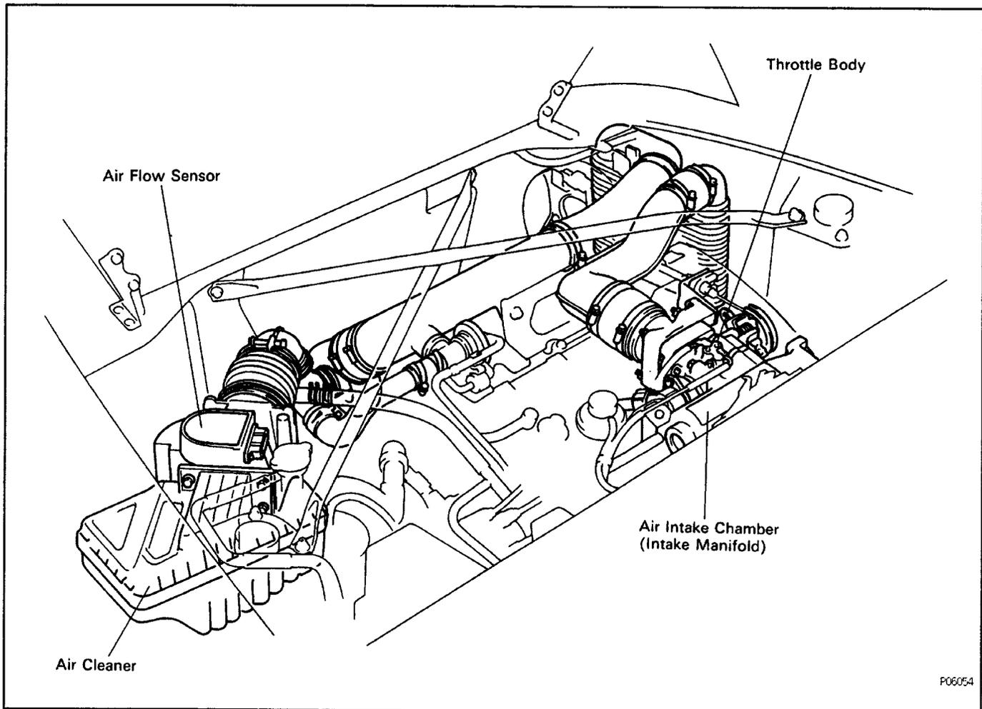
Air filtered through the air cleaner passes through the air flow sensor and the amount flowing to the air intake chamber is determined according to the throttle valve opening in the throttle body and the engine rpm.
