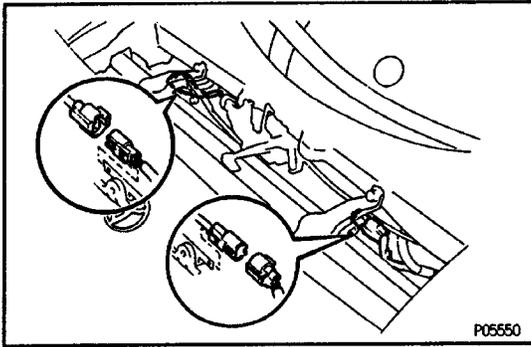
(b) Connect the two cooling fan connectors.
