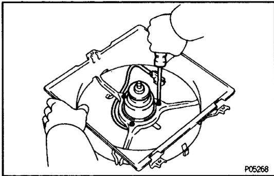
(b) Remove the three screws and fan motor.
