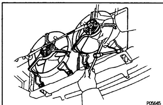
(b) Remove the three bolts and cooling fan. Remove the two cooling fans.
