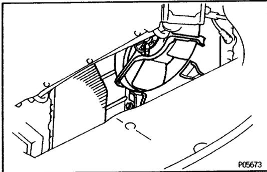
(b) Check that the cooling fan stops.
