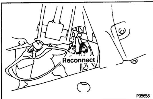
(e) Reconnect the engine coolant temperature switch.
