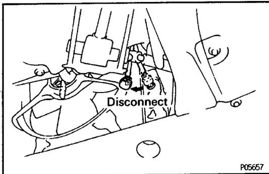
(c) Disconnect the engine coolant temperature switch.
