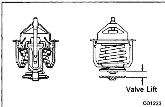
(c) Check the valve lift.
