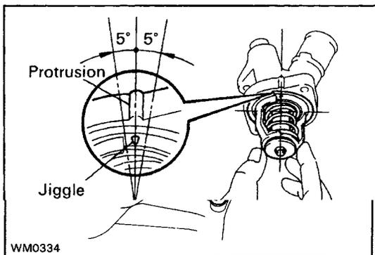
(b) Align the jiggle valve of the thermostat with the protrusion of the water inlet, and insert the thermostat in the water inlet.
