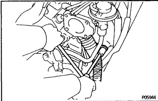
(c) Install the engine wire protector with the bolt.
