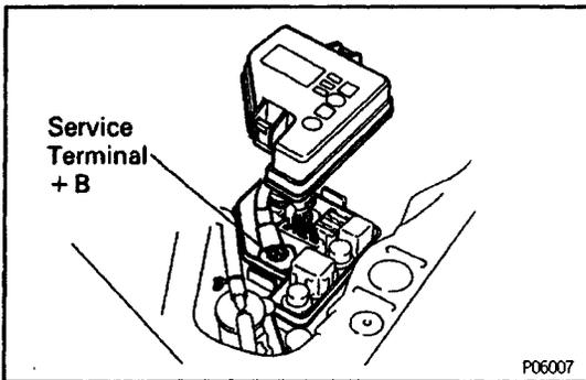
3. With a tachometer connected to the system, connect the power source probe of the tachometer to service terminal +B of the engine compartment relay box.
