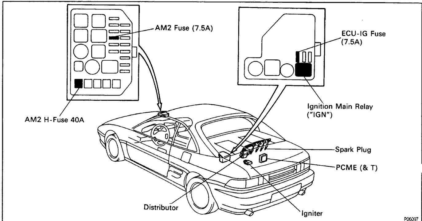
The PCME (& T) monitors the engine condition by signals from each sensor, calculates the ignition timing and sends an ignition signal to the igniter. High voltage from the ignition is distributed to each spark plug in the appropriate order to generate a spark between the electrodes, which ignites the air-fuel mixture.
