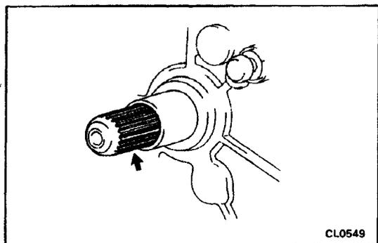
**5. APPLY SPLINE GREASE TO INPUT SHAFT SPLINE**
