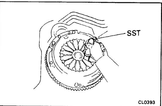
If alignment is not as specified, using SST, adjust the diaphragm spring tip alignment.
