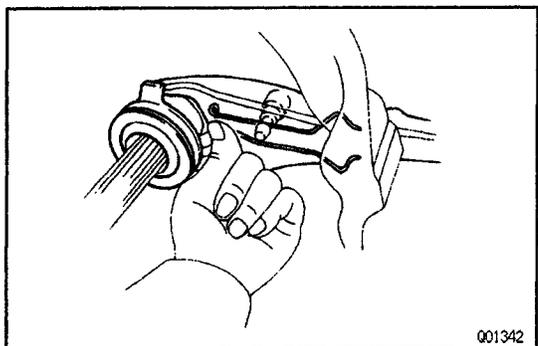
**6. INSTALL BOOT, FORK, HUB AND BEARING ON TRANSAXLE****7. INSTALL TRANSAXLE**
