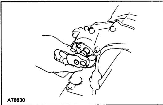
(b) Install a new O-ring to the sensor cover.
