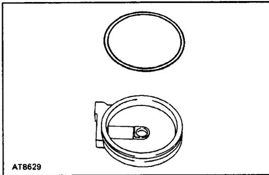
(c) Install the sensor cover to the transmission and then install the sensor cover bracket with the two bolts.
