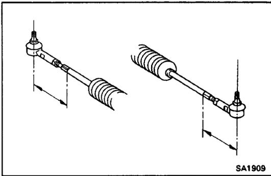
If wheel angles differ from the standard specifications, check to see if the lengths of the left and right tie rods are the same.
