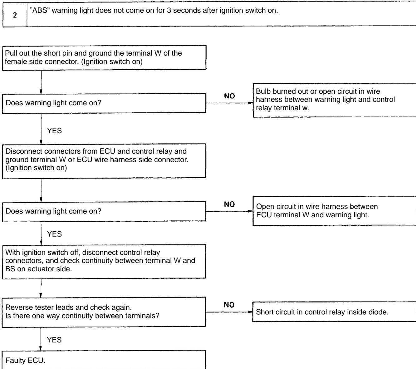
HINT: If the diode is short-circuited, a malfunction at ECU terminal W will occur. When inspecting the terminal, connect the ECU connector, and disconnect actuator connectors and data link connector. Then turn the ignition switch on, and check that the warning light goes on. If it does, the ECU terminal is OK.
