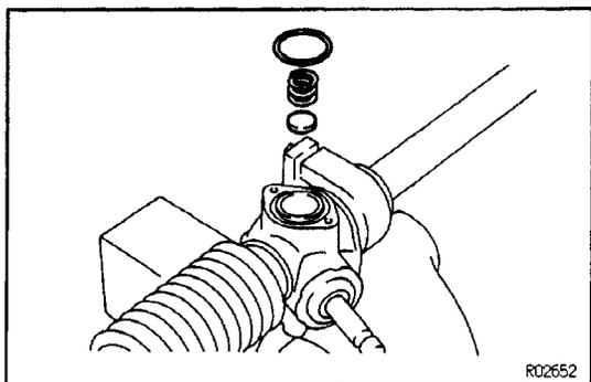
**9. INSTALL RACK GUIDE SPRING SPACER****10. INSTALL COMPRESSION SPRING****11. INSTALL O-RING**
