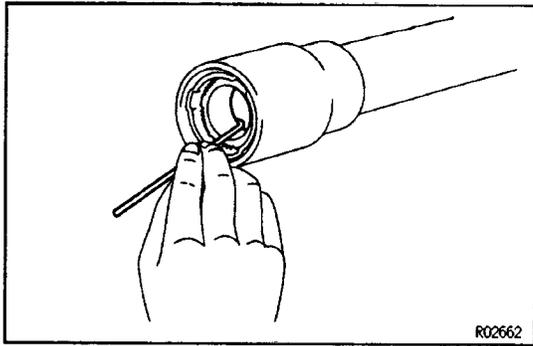
(b) Insure that the tube holes are not clogged with grease.
