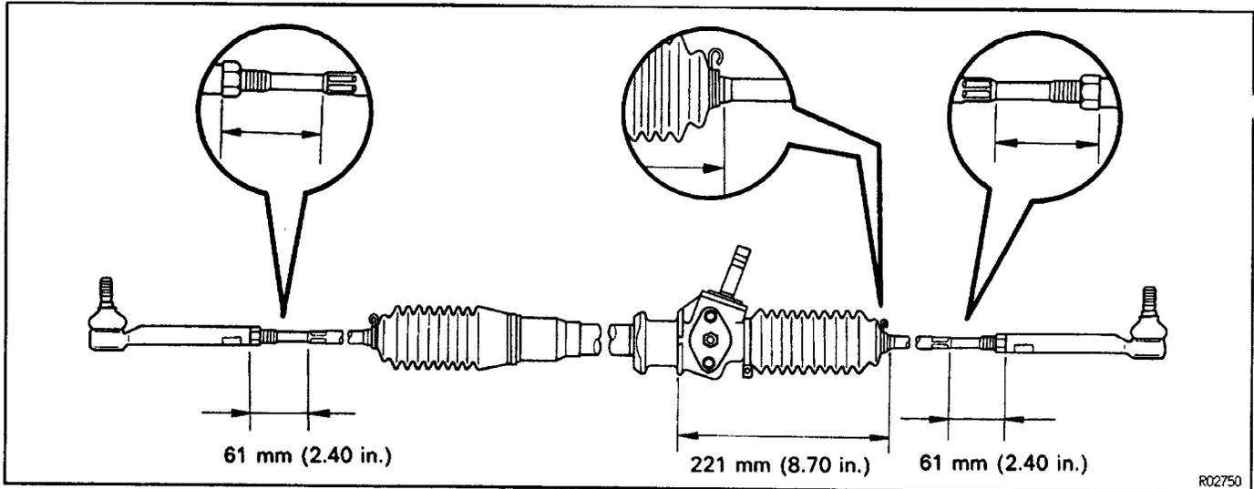
HINT: The dimension of the tie rod end is a reference value, so always adjust the toe-in before tightening the lock nut.
