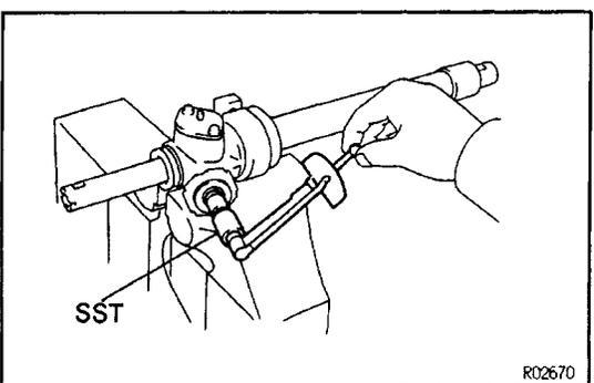
(b) Measure the total preload with SST.
