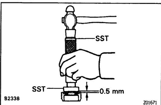
(b) Using SST, drive in a new oil seal until it is protruding 0.5 mm (0.020 in.)
