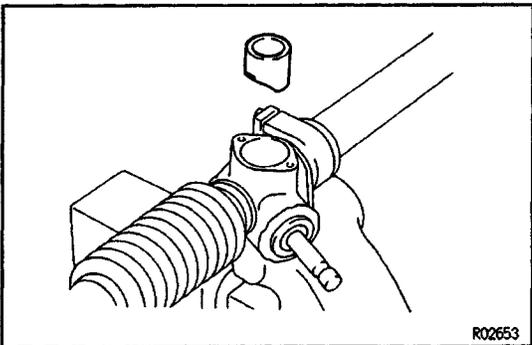
**11. REMOVE RACK GUIDE SUB-ASSY**
