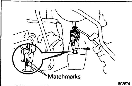
(b) Align matchmarks on the universal joint and pinion shaft and connect them.
