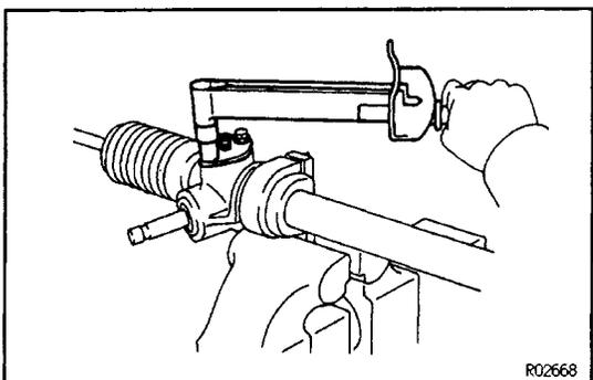
**12. INSTALL RACK GUIDE SPRING COVER SUB-ASSY**
