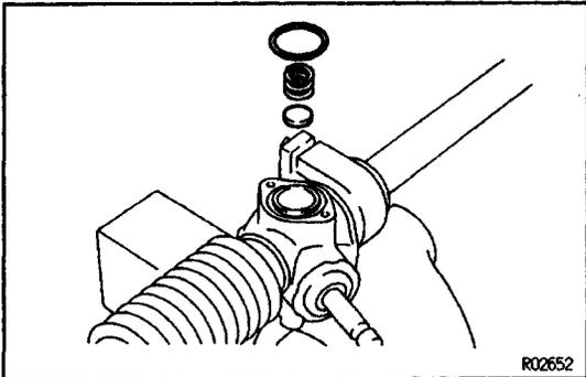
**8. REMOVE O - RING****9. REMOVE COMPRESSION SPRING****10. REMOVE RACK GUIDE SPRING SPACER**
