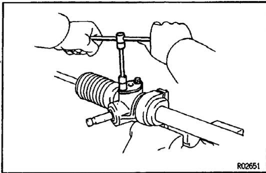
**7. REMOVE RACK GUIDE SPRING COVER SUB -ASSY**
