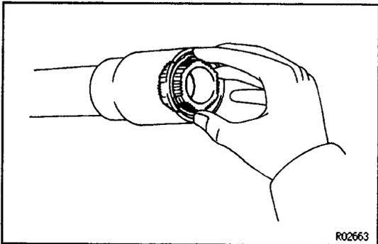
(c) Install a new bushing into the rack housing, making sure to align into the three holes.
