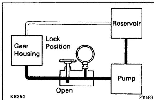
If pressure is low, the gear housing has an internal leak and must be repaired or replaced.
