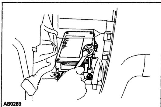
(b) Using a torx wrench, loosen and tighten the four screws.
