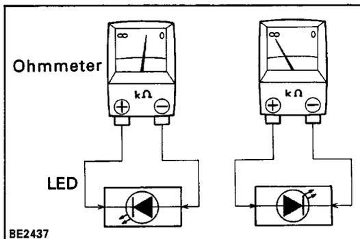
Check LED (Light Emitting Diode) in the same manner as that for diodes.
