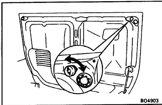
**3. ADJUST REAR EDGE OF ENGINE HOOD IN VERTICAL DIRECTION**
