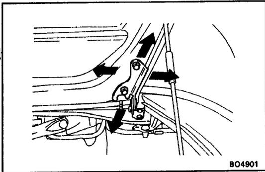
**1. ADJUST ENGINE HOOD IN FORWARD / REARWARD AND LEFT/RIGHT DIRECTIONS**
