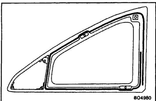
**2. APPLY ADHESIVE AT MOULDING INSTALLATION AREA**
