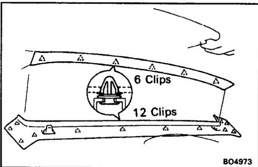
**10. INSTALL ROOM PARTITION TRIM MOULDING****11. INSTALL ROOF HEADLINING REAR TRIM****12. INSTALL DOOR SCUFF PLATE**
