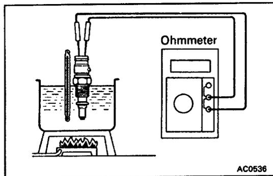
If resistance value is not as specified, replace the sensor.
