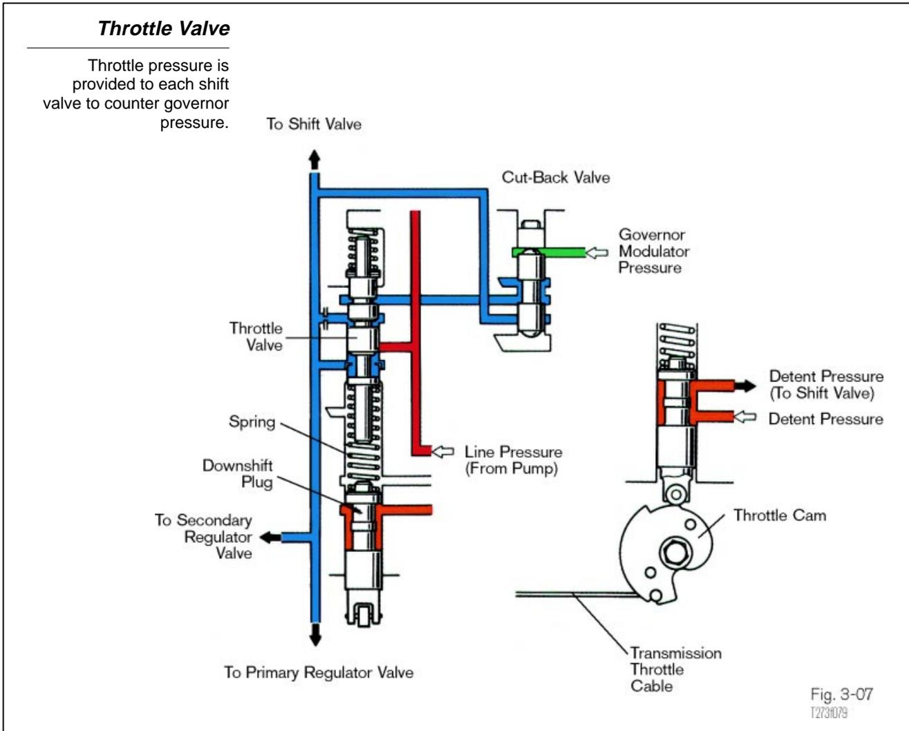
**Shift Control Valves** Shift control valves are responsible for directing fluid to different passages in the transmission. They can be manually controlled, solenoid controlled, or hydraulically controlled. They block hydraulic passages while other lands of the valve open passages.
