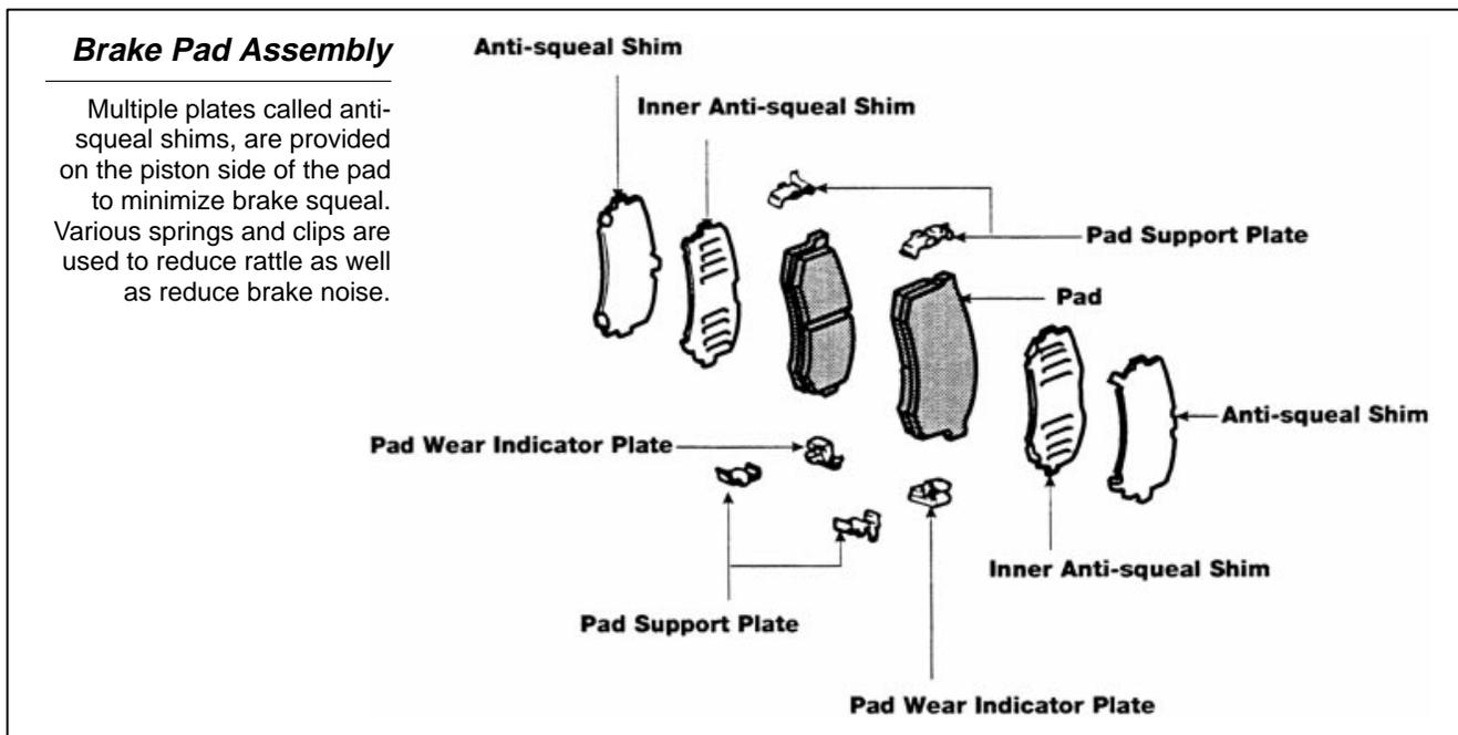
The brake pad material is bonded to a stamped steel backing plate with a high temperature adhesive to which heat and pressure are applied to cure the assembly. A slit is provided on the face of the pad to indicate the allowable limit of pad wear and provide a path for brake dust and gas to escape.
