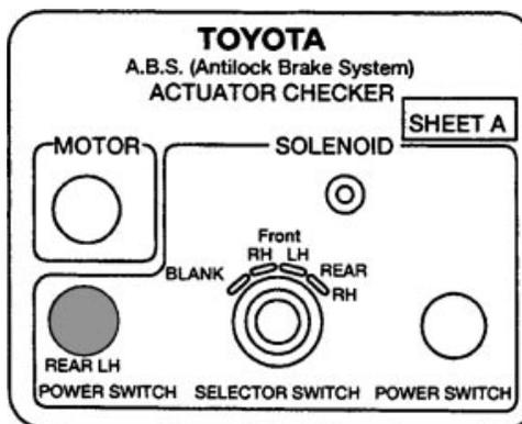
The ABS actuator checker statically checks the operation of the actuator which includes: the pump, solenoids, and relays. If a normal code is displayed, but symptoms still occur, refer to the Problem Symptoms Chart in the Repair Manual. The chart indicates when the checker is to be used.
