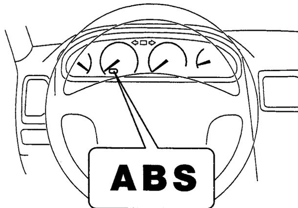
**Trouble Code Check** To access the diagnostic trouble codes stored in the ECU, locate the Data Link Connector (DLC1) or (DLC2). Consult the Repair Manual or the ABS Reference Card to determine whether the ABS Check Connector is physically disconnected or the short pin for Wa and Wb is removed.
