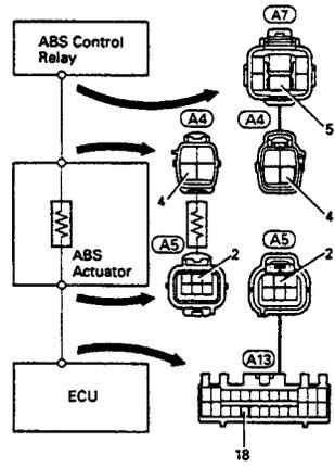
**P** Disconnect the 2 connectors from ABS actuator.
