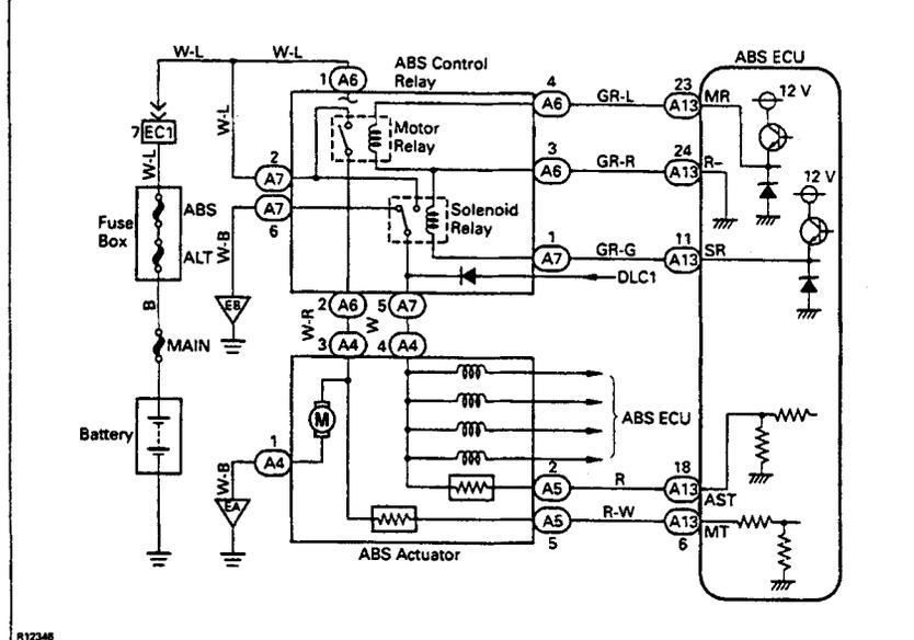
An inspection procedure follows the circuit inspection with components, connectors, pin locations and measurement values to diagnose the circuit. Each step is outlined in sequence, leading to a repair.
