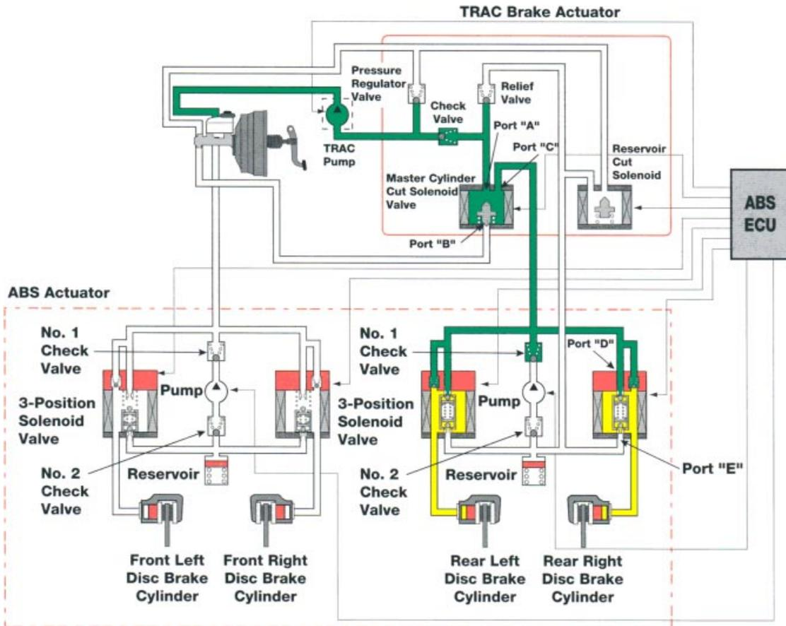
**Pressure Reduction Mode** When decreasing pressure applied to the rear brake cylinders, the ABS ECU engages the 3-position solenoid valve in the ABS actuator to the pressure reduction mode. Fluid pressure applied to the brake cylinder returns to the master cylinder reservoir from the 3-position solenoid valve and reservoir in the ABS actuator to the Reservoir Cut Solenoid Valve, thus alleviating the brake fluid pressure.
