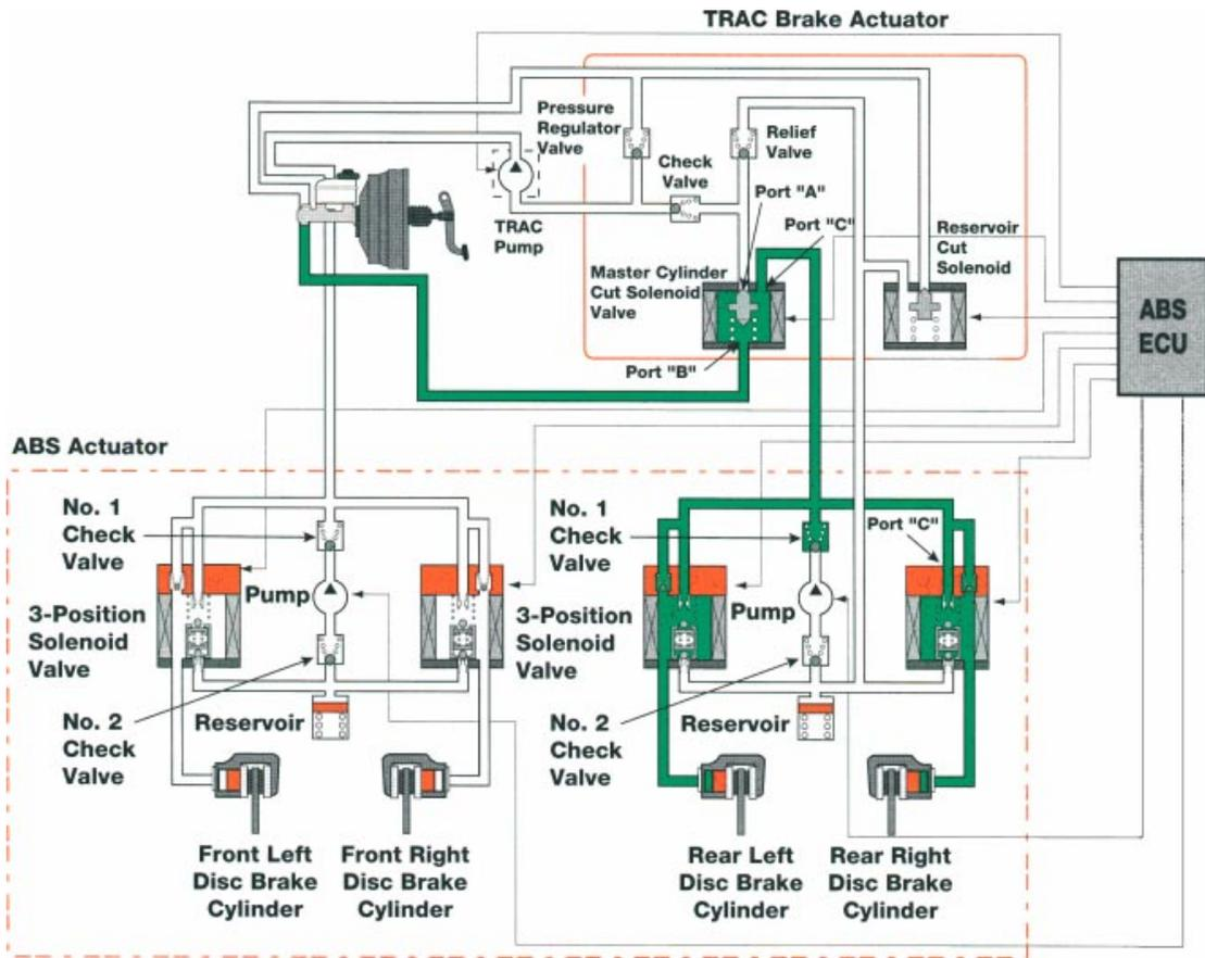
**TRAC Operation** Dialing normal operation (TRAC not activated) all solenoid valves of the TRAC brake actuator remain inactive when the brakes are applied. As the brake pedal is depressed, brake fluid pressure generated by the master cylinder is applied to the disc brake cylinders, via the master cylinder cut solenoid valve, and the 3-position solenoid valves in the ABS actuator. When the brake pedal is released, fluid pressure returns from the disc brake cylinders to the master cylinder.
