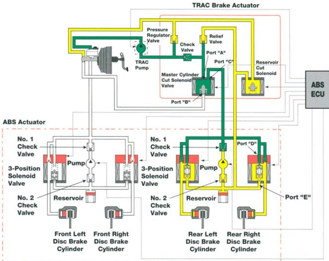
**Wheel Speed Control** The TRAC ECU constantly receives signals from the 4 speed sensors and calculates the speed of each wheel. At the same time, it estimates the vehicle speed based on the speed of the 2 front wheels and sets a target control speed.
