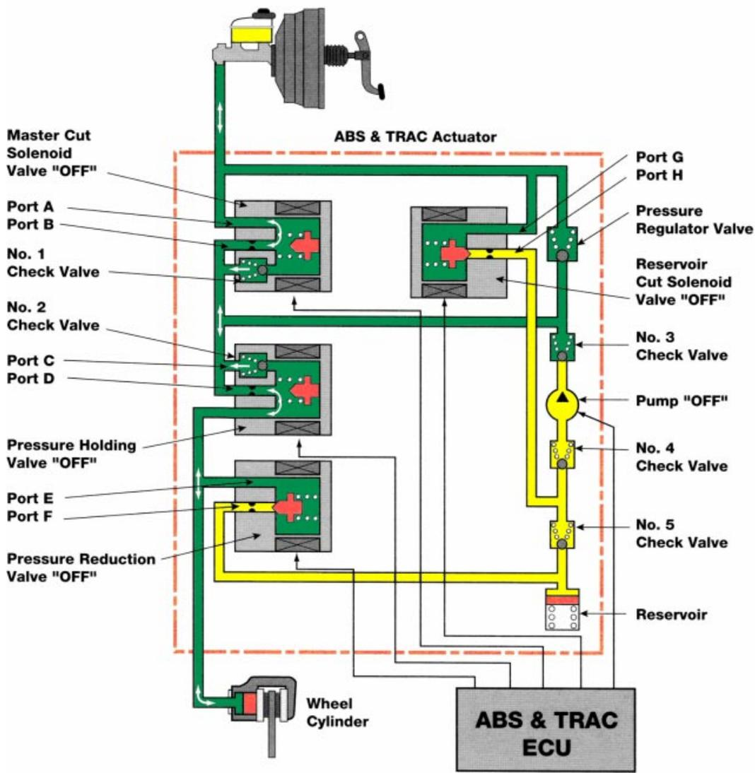
**Pressure Increase Mode** During sudden acceleration or driving on a slippery surface, if the drive wheels start to slip the ABS & TRAC ECU causes the actuator to go into pressure increase mode.
