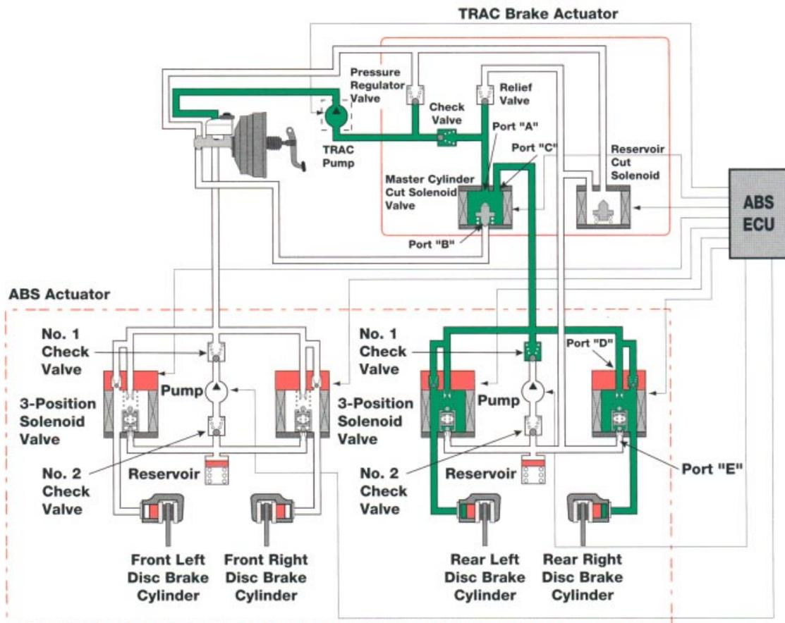
**Pressure Holding Mode** When the brake fluid pressure for the rear brake cylinders is increased or decreased as required, the system switches to the holding mode. This mode change is performed by engaging the 3-position solenoid valve in the ABS actuator to the holding mode. This results in blocking the TRAC pump pressure from flowing to the disc brake cylinder through port D.
