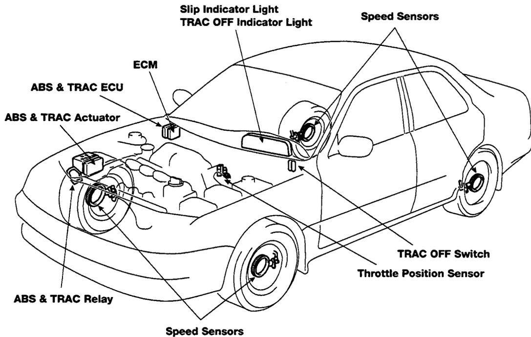
**Camry/Avalon TRAC** The ABS/TRAC ECU and ECM work together to provide traction control. The ABS/TRAC/ECU monitor signals from the four speed sensors to determine the speed of each wheel and vehicle speed. When slippage is determined:
