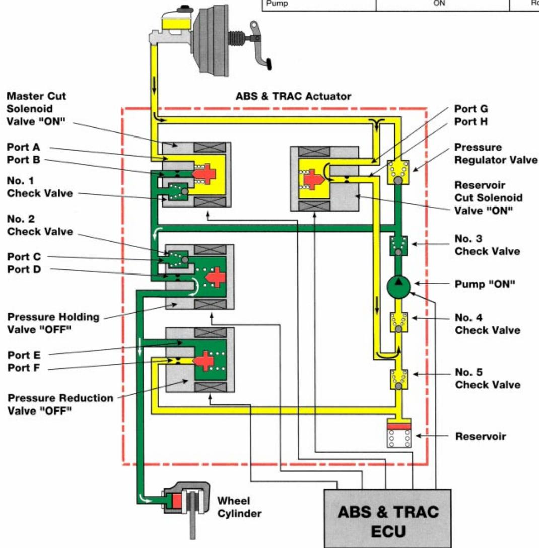
**Pressure Holding Mode** When fluid pressure in the wheel cylinder circuit is optimized by an increase or decrease in pressure, the ABS & TRAC ECU controls the system as follows:
