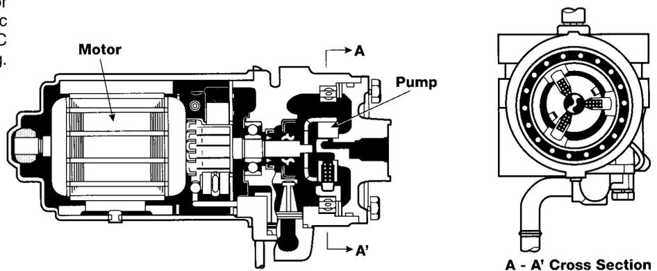
**TRAC Brake Actuator** The **TRAC Brake Actuator** consists of two cut solenoid valves and three spring loaded valves which regulate the brake fluid pressure in the right and left rear wheels. The rear wheels are controlled independently through the ABS actuator based on signals from the ABS ECU.
