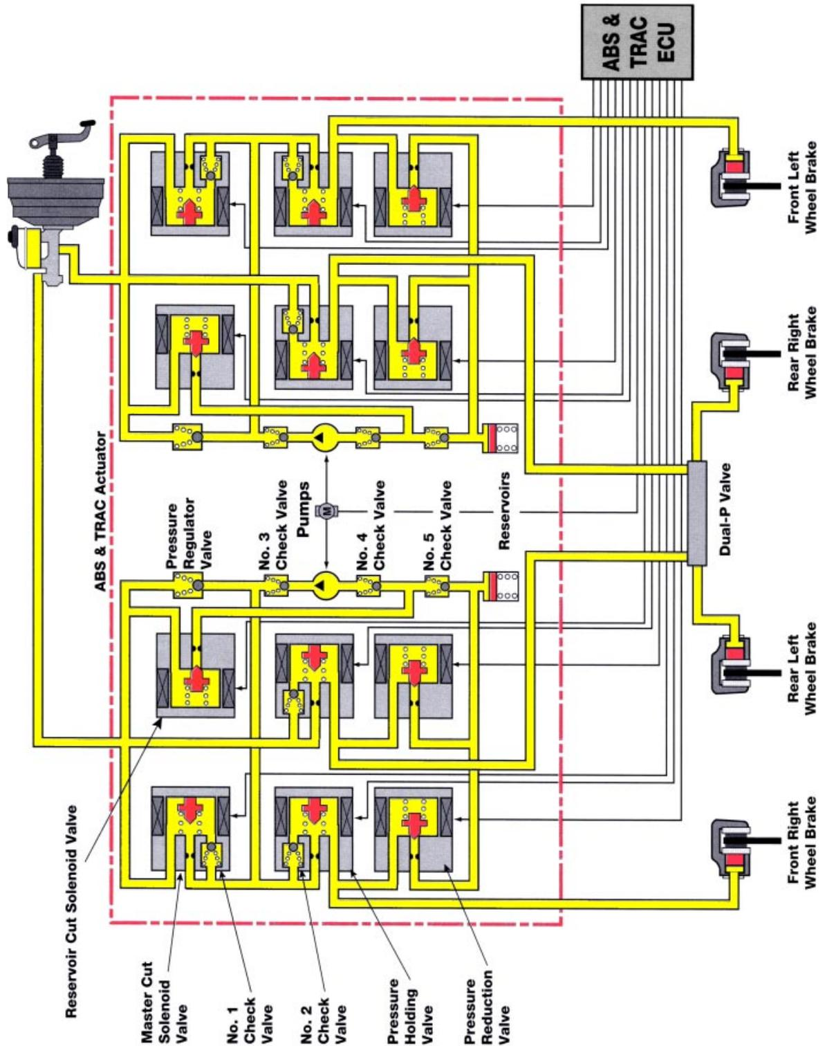
**Normal Operation Mode** During normal operation when the TRAC system is not activated all actuator valves are OFF. The Master Cut Solenoid Valve is open allowing fluid from the master cylinder to flow through the Pressure Holding Valve to the wheel cylinder. In this mode the brakes function just like a system without ABS or TRAC.
