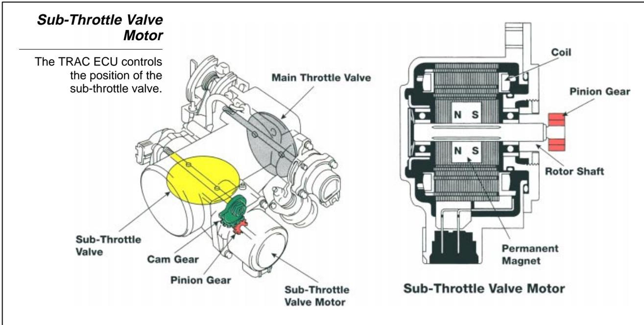
The sub-throttle valve motor consists of a permanent magnet, a coil, a rotor shaft and pinion gear. It is a step motor that is rotated by a signal from the ABS & TRAC ECU. The pinion gear rotates a cam gear, fitted on the sub-throttle valve shaft end, controlling the sub-throttle valve opening angle.
