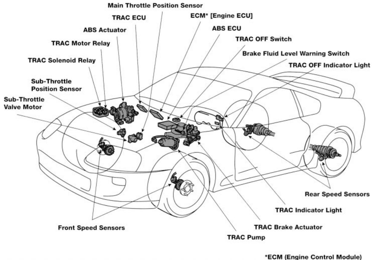
**Operation Of Components** The TRAC OFF switch is located on the instrument panel above the center console. It allows the driver to activate or deactivate the TRAC system when the switch is depressed. The system defaults to ON when the ignition switch is cycled.
