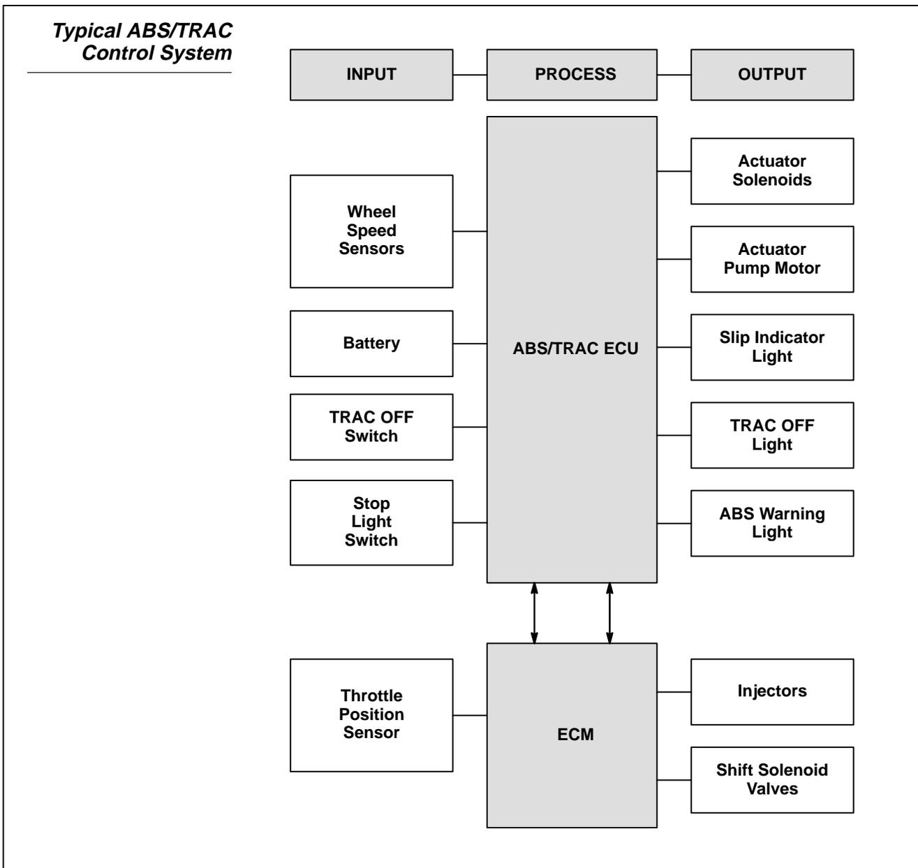
Wheel Speed Control Wheel speed control is accomplished by two means:
