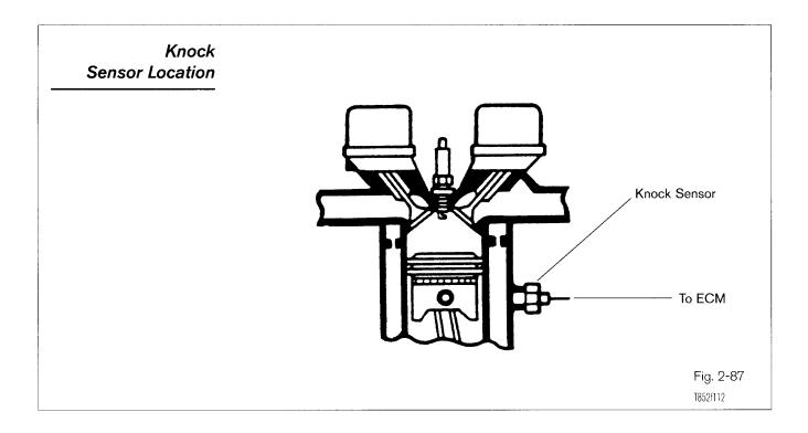
Inside the knock sensor is a piezoelectric element. Piezoelectric elements generate a voltage when pressure or a vibration is applied to them. The piezoelectric element in the knock sensor is tuned to the engine knock frequency.
