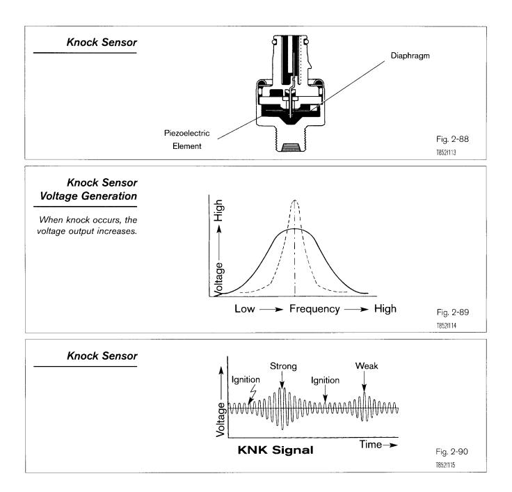
The vibrations from engine knocking vibrate the piezoelectric element generating a voltage. The voltage output from the Knock Sensor is highest at this time.
