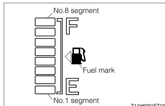
3. Short-circuit the vehicle harness side connector terminals 1 and 2 of the fuel sender gauge.
