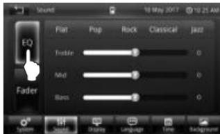
Touch [**Fader**] to display the sound balance & fader control screen. Move the cursor to adjust the required balance & fader sound position.
