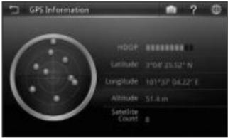
3. Screen will display the position of GPS satellites, latitude, longitude, altitude, satellite count and HDOP bars **at your current location**.
