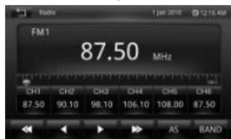
**[▶]** Press to tune the frequency up manually.
