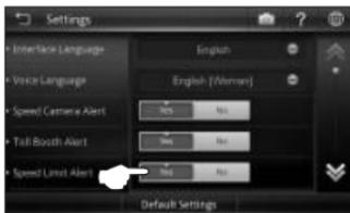
2. Select **Yes** to enable the system to provide voice prompt whenever the car exceeded the speed limit.
