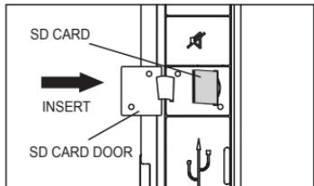
Removing the SD card from the unit will also stop play back.
